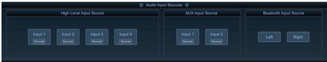
3)Each output channel can be added to the Analog input sourceby dragging the mouse or double-clicking with the left button.Users can add inputs by drawing them( IN1~IN4) to the output channels, axis or double click them with left button of the mouse.
