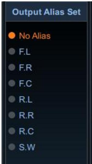
2)After aliasing the output channels, you will be prompted to load the filter preset value or not. If you select yes, the filter preset value will be loaded automatically:Butterworth@12dB/Oct. (Full range:0~20KHz, High range:3K~20KHz, Middle range:500~3KHz, low range:20~500Hz, Subwoofer:20~80Hz)
