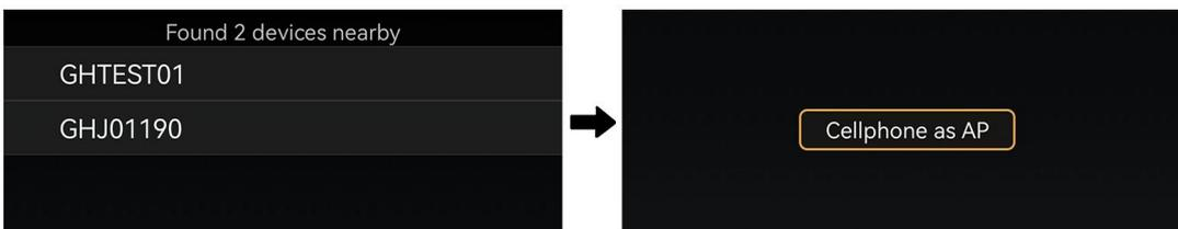
1) Enter the [Hotspot Name] and [Hotspot Password], click [OK], select [Open Hotspot Settings] to enter the phone hotspot setting interface, and turn on the phone hotspot. Finally, return to the app and wait patiently for a moment to complete the connection.
